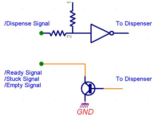
Figure 3: TTL Logical Diagram
