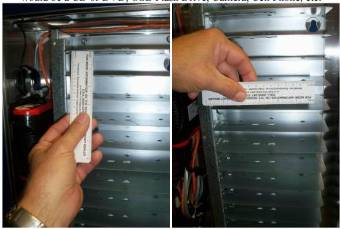
7. The shelves can be dropped by moving the side bar back and forth on the left side of the machine.
