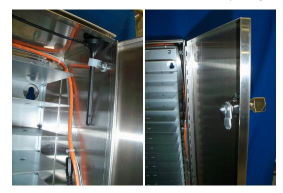
5. Note the Verizon Cellular Antenna is mounted inside the cabinet & secured by a 90 degree cam lock.
